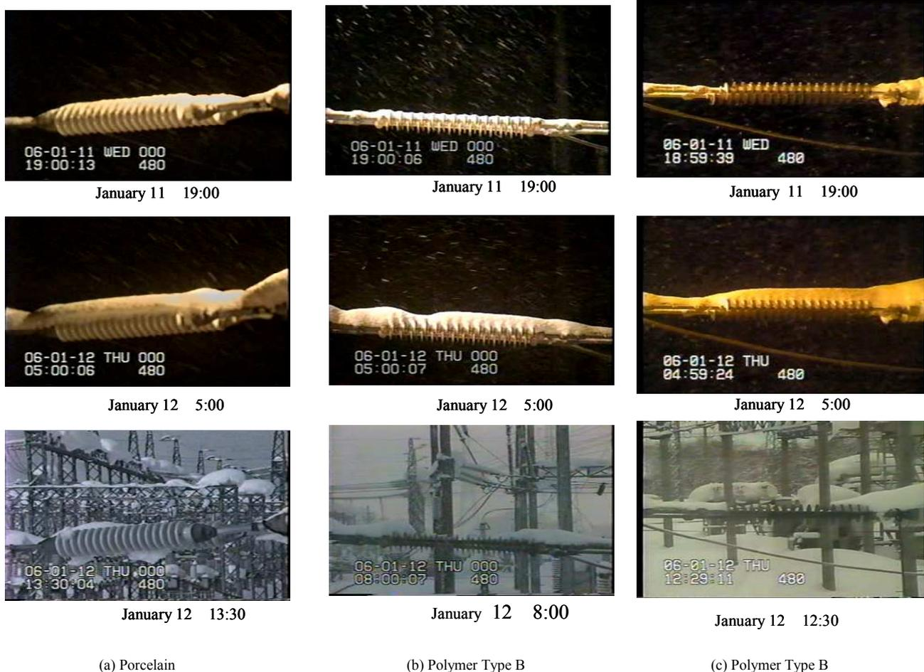
Fig. 2. Capped snow formed on three kinds of long rod insulators.
