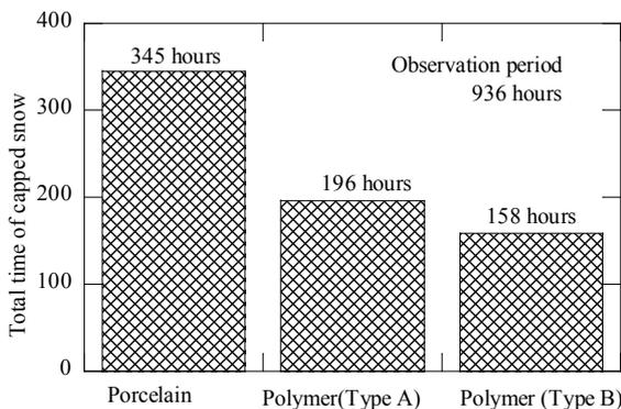
Fig. 6. The total time of capped snow on the insulators.
