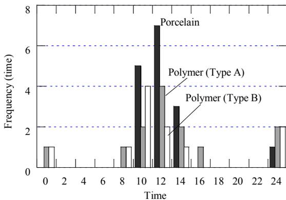
Fig. 5. The occurrence frequency of drop-off time of capped snow.
