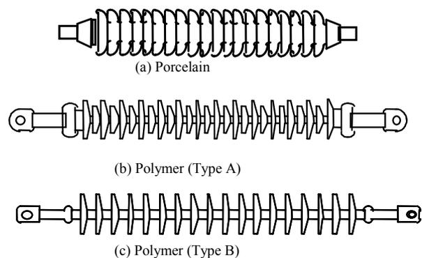
Fig. 1. Shapes of three rod-type insulators.
